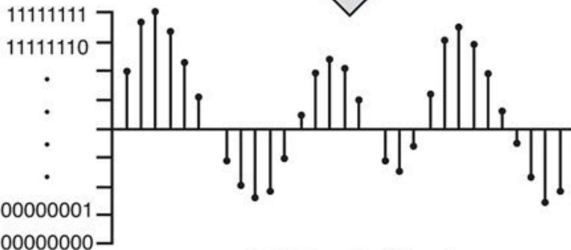
PCM Encoded Signal
